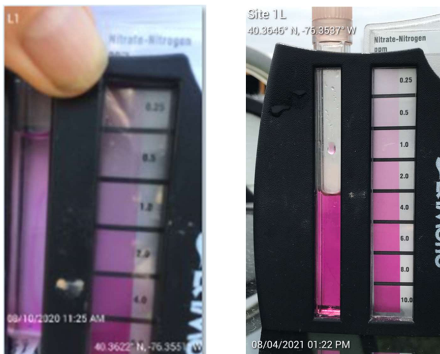
Photo 1 – Comparison of Nitrate LaMotte Test Kit Color Results - 2020 vs 2021
